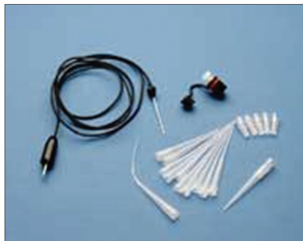
Figure 2: Electrodes used for the preparation of KCL-agar electrodes
